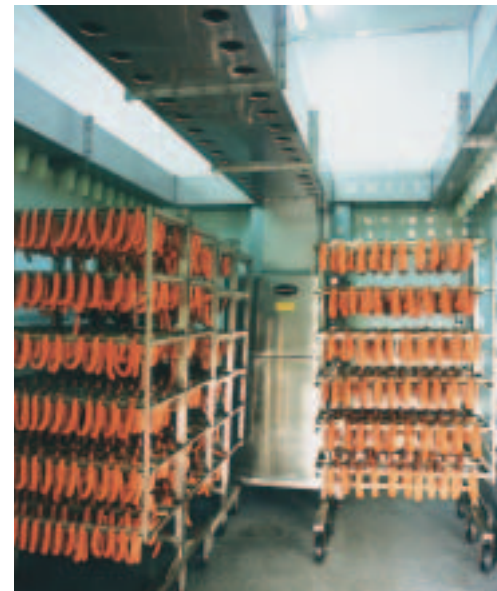
CLIMASTAR KNR: Air conditioned post maturing facility for 20 trolleys
