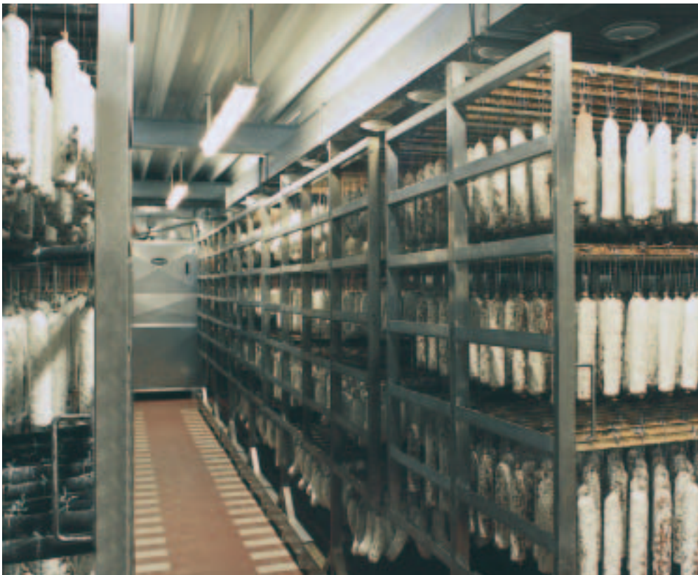
CLIMASTAR KNR – air conditioned curing facility for 60 trolleys
